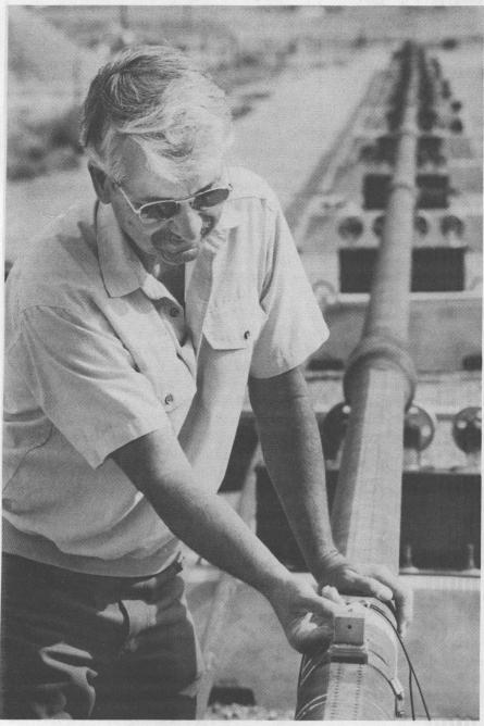
ORPHEUS RANGE — Doug Drumheller (6111) checks an accelerometer used to measure motion along 1,500 feet of steel drilling pipe at Orpheus Range in Tech Area 3. The horizontally mounted pipe at the range is being used for a number of drilling projects, including efforts to improve transmission of data by sound waves from deep within a well.
